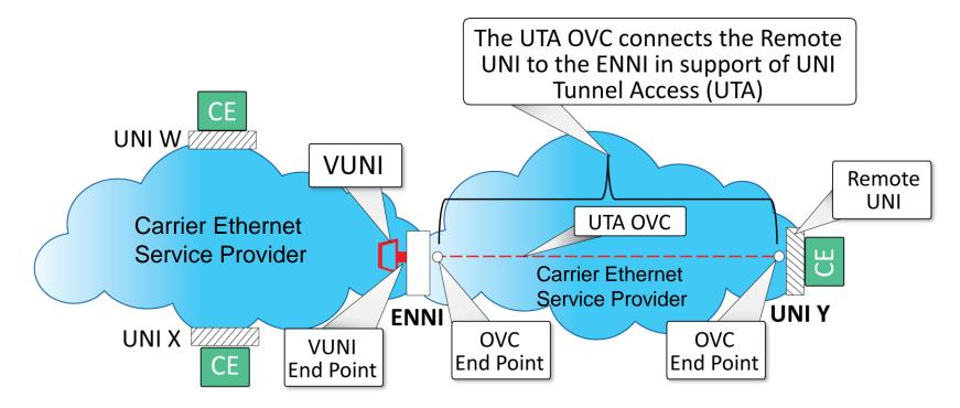
Network Operator provides the OVC for transfer of Service Frames between the remote UNI and the ENNI.
